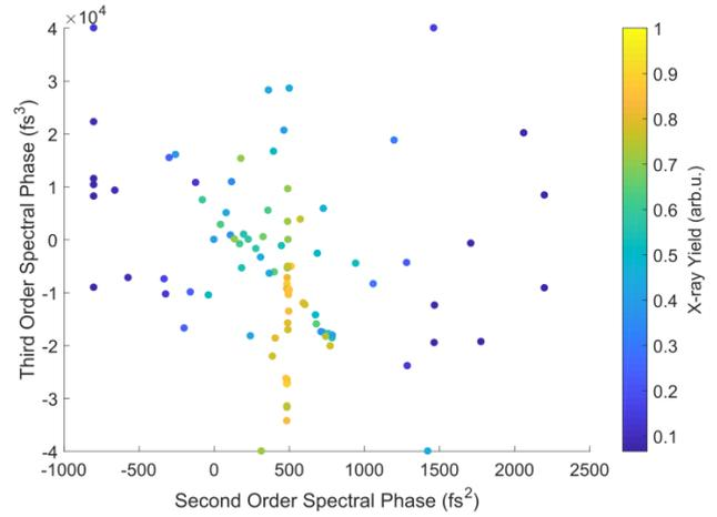
Figure 2: Every trial solution attempted by the genetic algorithm across all generations, with the colour representing the x-ray yield of each trial solution.
