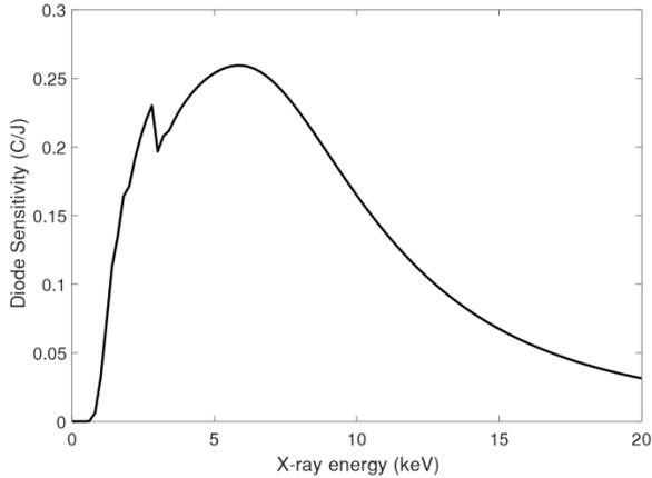
Figure 1: Sensitivity curve of the x-ray PIN diode, the transmission of its layered filter was also included in the calculation of this curve.
