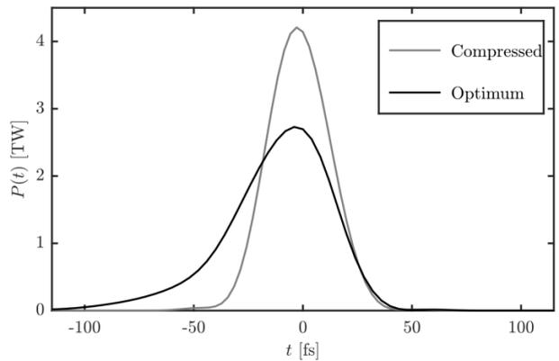
Figure 3: Temporal shape of the optimum pulse (found by the genetic algorithm) and the most compressed pulse.
